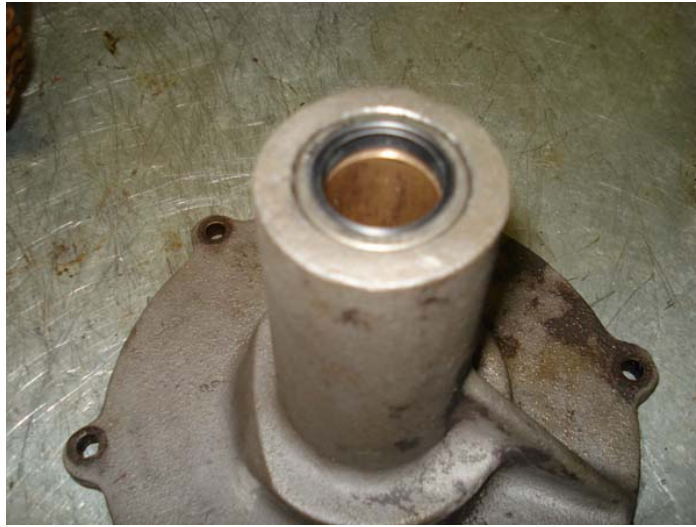
Drive in new Rear Axle Oil Seals.
